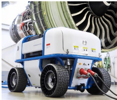
GE’s 360 Foam Wash is an alternative to water wash for engine maintenance © GE Aerospace
